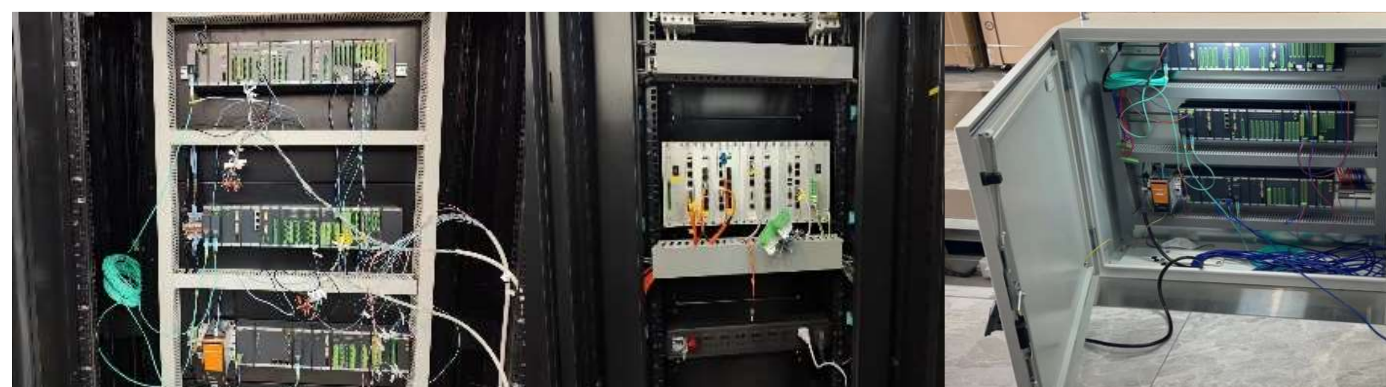
Fig. 4. Wind turbine main control, converter controller, wind farm station level controller, HVDC control protection device hardware in the loop.
